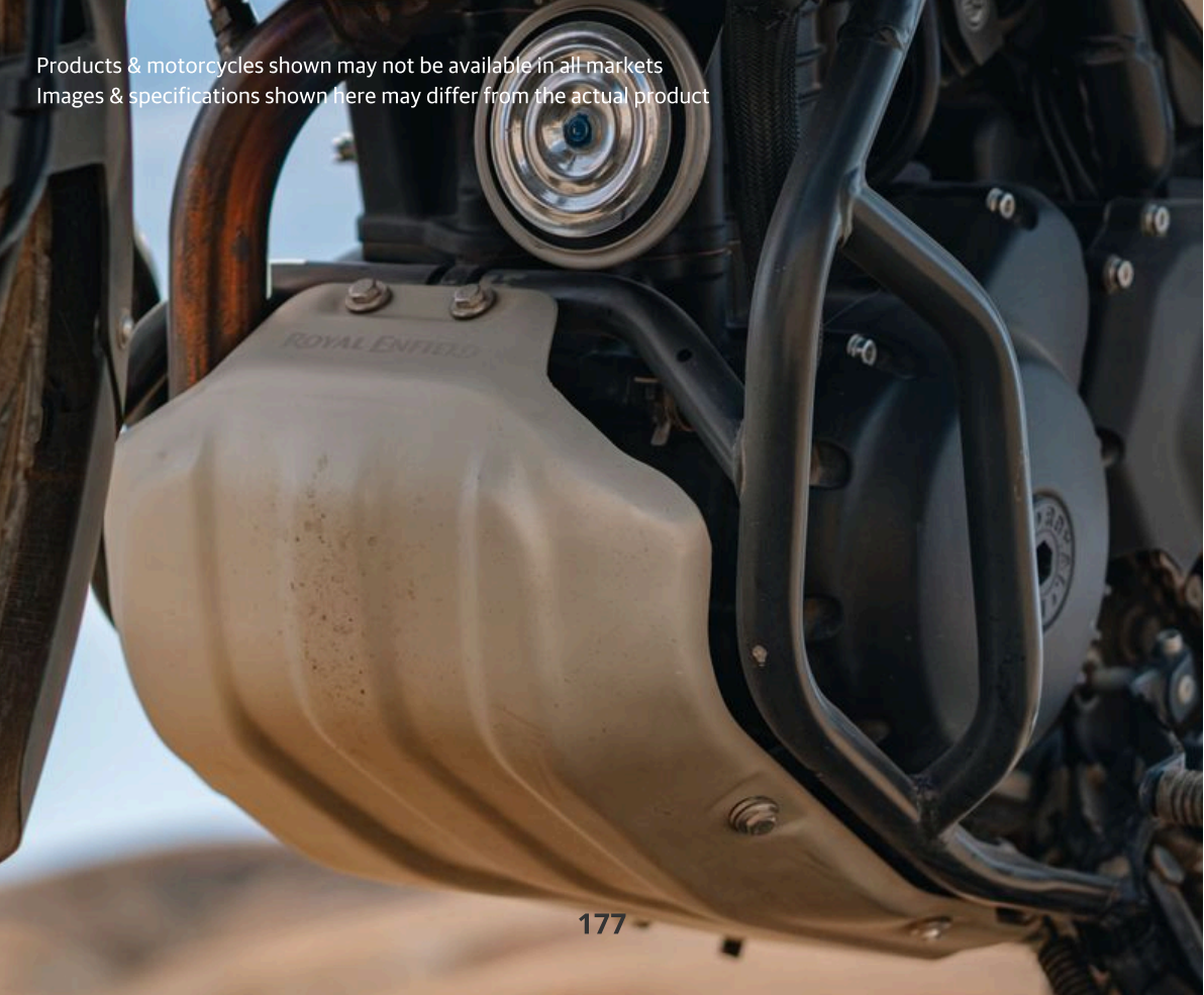
Tubular framework & brushed aluminium sumpguard Offers Maximum protection
